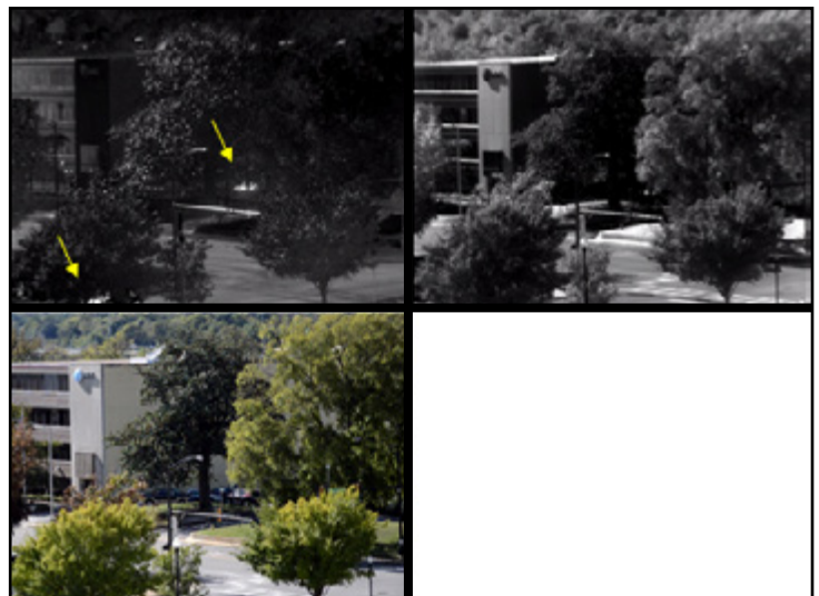
SWIR DoLP (upper left) shows cars partially obscured and in heavy shadow that are not seen in the SWIR S_0 image (upper right) or VIS S_0 image (lower left).
