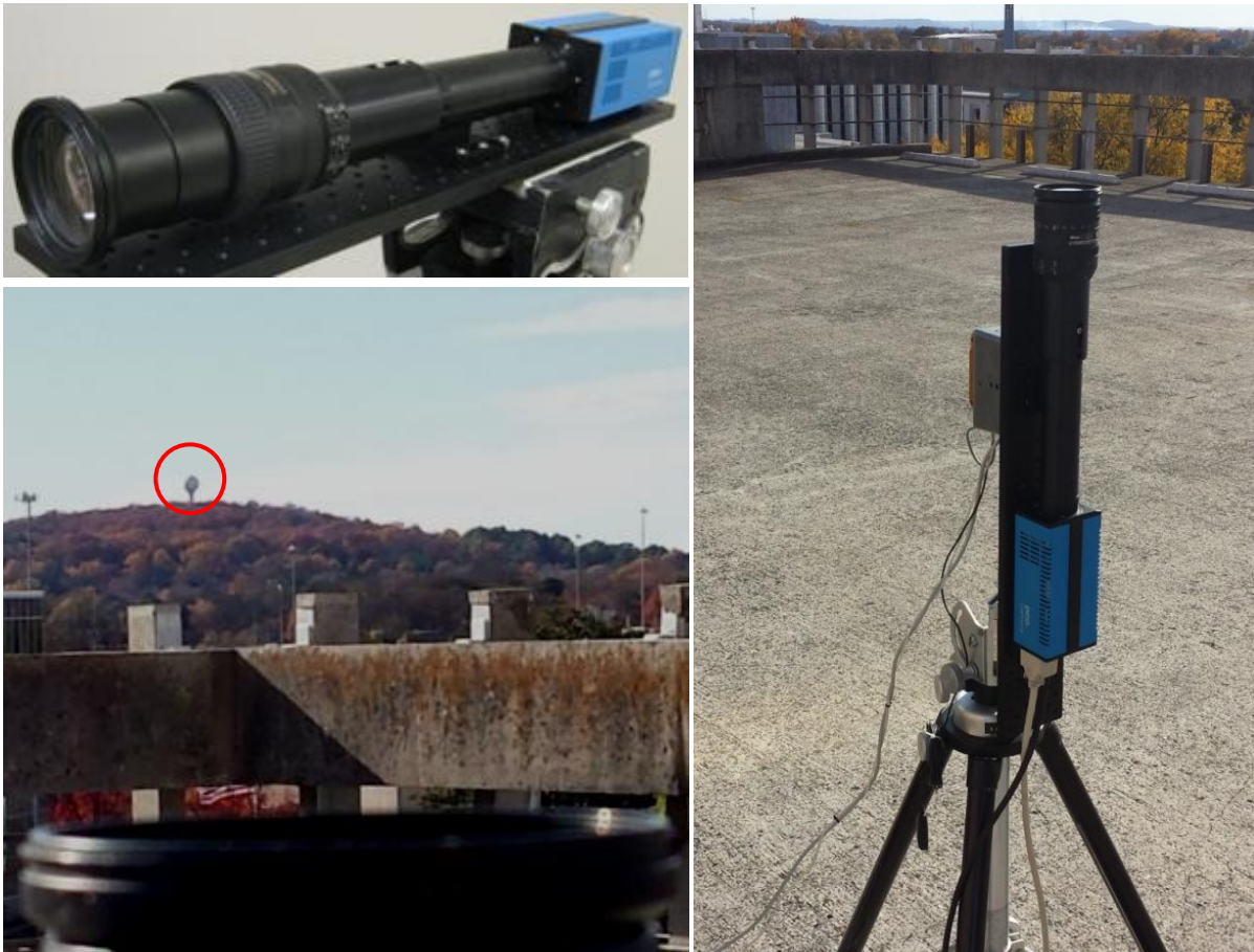
Figure 6. Photographs of the imaging polarimeter (top left), the polarimeter in operation (right), and a view across the objective at the water tower used for orienting the sensor (red circle).
