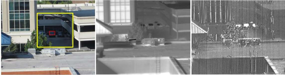
Figure 4. Vehicles at thermal equilibrium with surroundings shown in the visible reference image (left), standard thermal image (middle), and polarimetric image (right).
