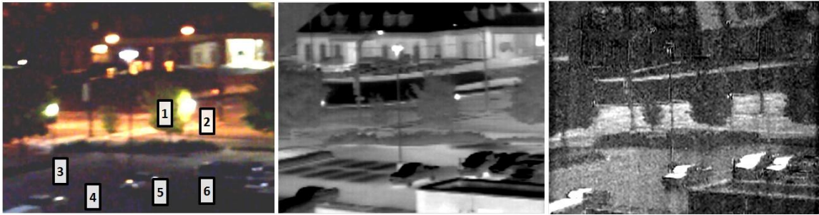
Figure 9. Recovery of contrast in polarimetric image in low light conditions illustrated in the visible reference image (left), standard thermal image (middle), and polarimetric image (right).
