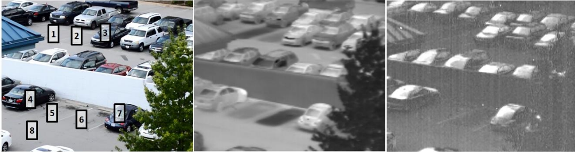
Figure 5. Mitigation of thermal shadows using polarimetry illustrated in the visible reference image (left), standard thermal image (middle), and polarimetric image (right).
