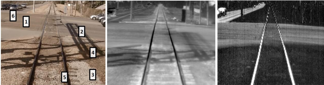
Figure 8. Shadow extended across train tracks and roadway shown in the visible reference image (left), standard thermal image (middle), and polarimetric image (right).
