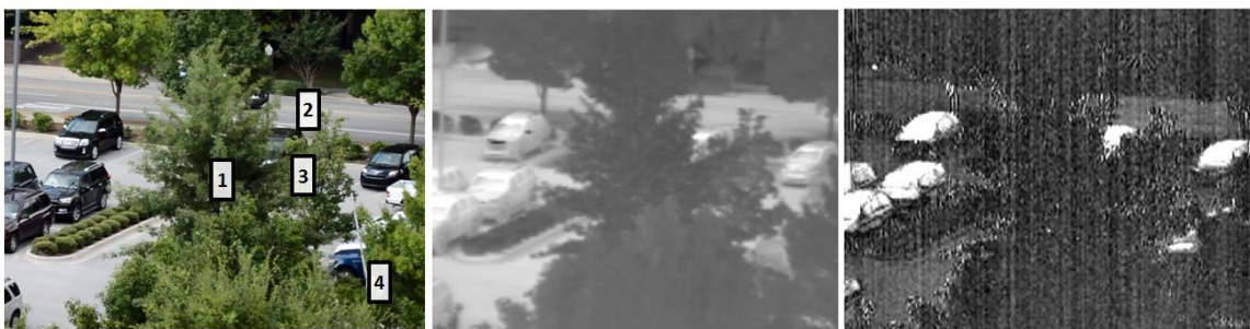
Figure 7. Detection of vehicles obscured by trees illustrated in the visible reference image (left), standard thermal image (middle), and polarimetric image (right).
