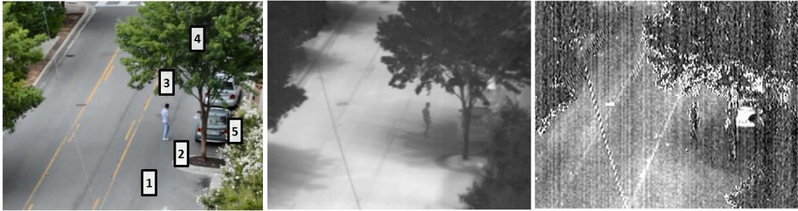
Figure 6. Pedestrian and vehicle in shadow shown in the visible reference image (left), standard thermal image (middle), and polarimetric image (right).
