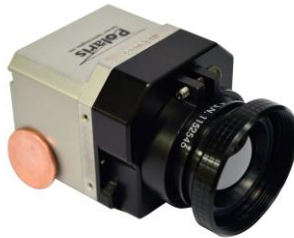
Figure 1. A Pyxis ® camera incorporates a micro filter array mounted in close contact to the COTS FPA.
