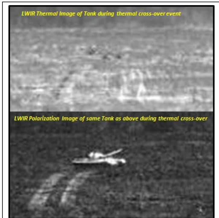
Figure 1 Comparison of a thermal LWIR image to LWIR polarimetric image during a thermal cross-over event.
