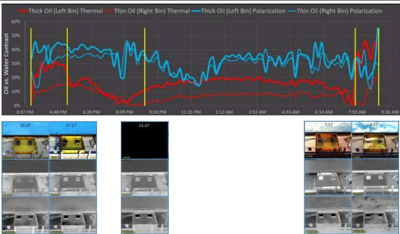
**Figure 1.** The plot shows Contrast computed for thermal (red) and polarization (blue) data products. Polarization performs better 92% of the time. The bottom imagery shows visible, thermal, and polarization imagery of the 5 mm thick (left bin, thick line in the plot) and 0.5 mm thick (right bin, thin line) oil samples at the times marked by yellow lines.
