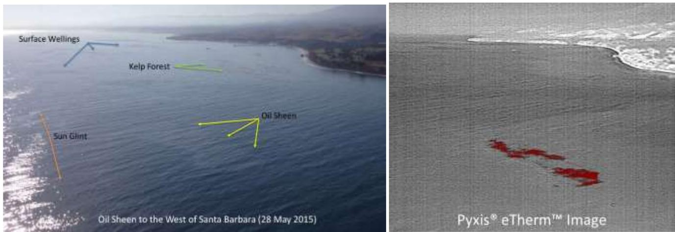
**Figure 3.** Oil spill detection off the coast of California. The Pyxis eTherm image shows the detection in red whereas the thermal and visible imagery show confusing clutter.
