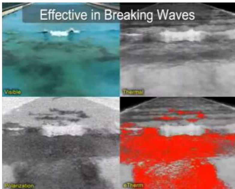
**Figure 2.** Visible, thermal, polarization, and eTherm imagery of crude oil on water in breaking waves. Oil is essentially undetectable in the thermal imagery.
