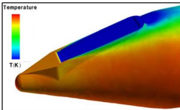
Hypersonic flight's significant thermal effects on the seeker window
