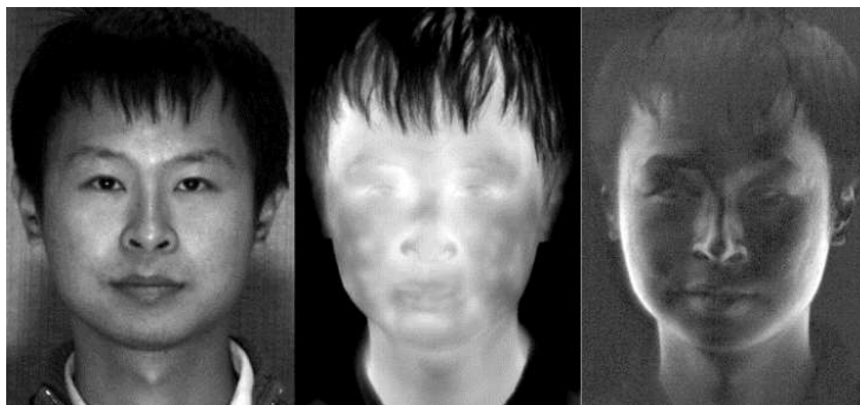
Figure 12. Visible (left), thermal infrared (center), and IR Polarimetric images (right). The polarimetric image shows detail around the eyes, nose, and mouth with clarity approaching that of the visible image. This imagery was taken with a cooled thermal camera.
