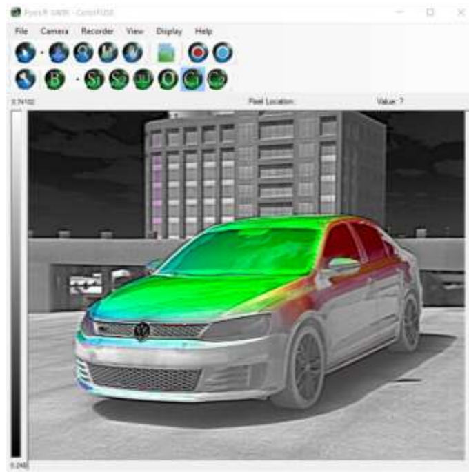
Figure 9. The Pyxis® Vision Science user interface main window. The first row of buttons below the menu are tools to manipulate the image. The second row of buttons select the quantity displayed: radiance, Stokes vector elements S1 and S2, degree of linear polarization, orientation, and ColorFuse data. ColorFuse display of polarization is shown.
