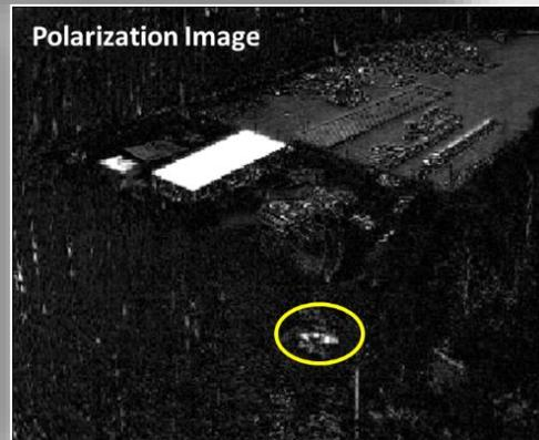
Using Polaris's polarimetric cameras, the DoD agencies have demonstrated that thermal polarimetric detection is effective for detection of man-made, surface-laid targets, aerial targets, and mobile targets. Polarimetric detection is specifically beneficial when the target and background are close to thermal equilibrium or when the background is highly cluttered.
