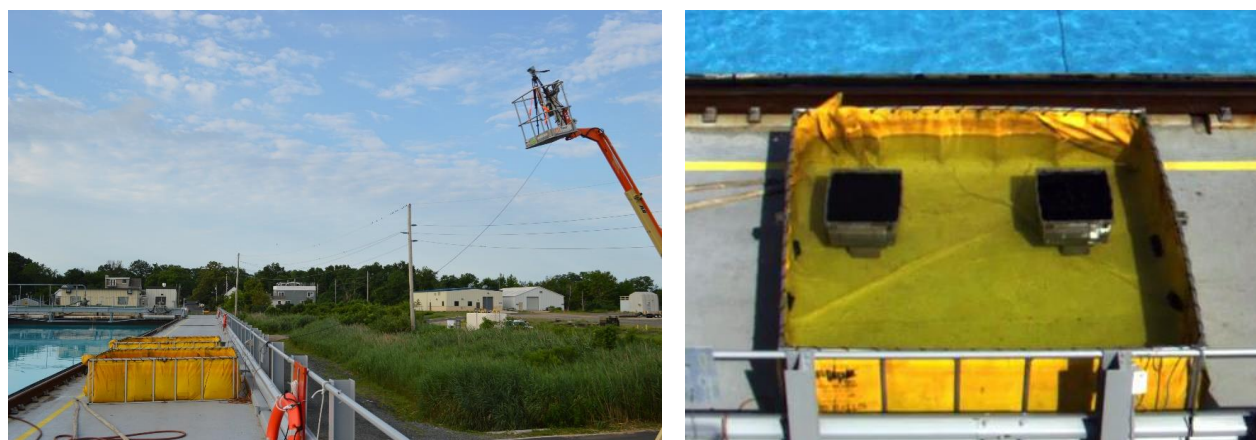
Figure 7. “Fast tank” test setup for thickness, angle, and overnight testing. The view on the right shows a close up of the bins viewed by the sensor placed on the man lift. The bin on the left was filled with water and 1000 mL of oil resulting in an oil thickness of 5 mm and the bin on the right was filled with water and 100 mL of oil giving a thickness of 0.5 mm. The water level in the fast tank was just below that of the lip of the bin to keep a fairly pristine water background for comparison.
