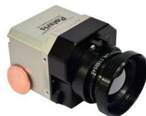
Figure 2. A Pyxis camera incorporates a micro filter array mounted in close contact to the COTS FPA.
