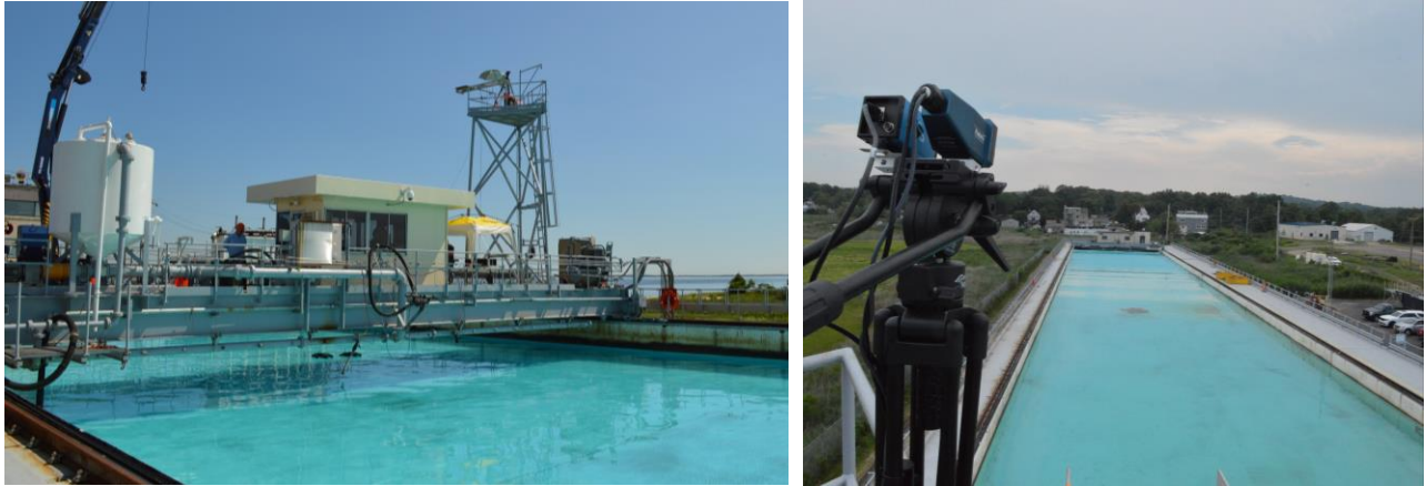
Figure 9. The moveable bridge over the Ohmsett tank. The Pyxis and visible camera were mounted on the tower at the right end of the bridge. The picture on the right shows the Pyxis and visible camera viewing the tank. Two small spills are visible about halfway down the tank. The wave machine was just started and the waves have almost propagated to the spills. The yellow fast tank is visible on the deck to the right side of the tank.
