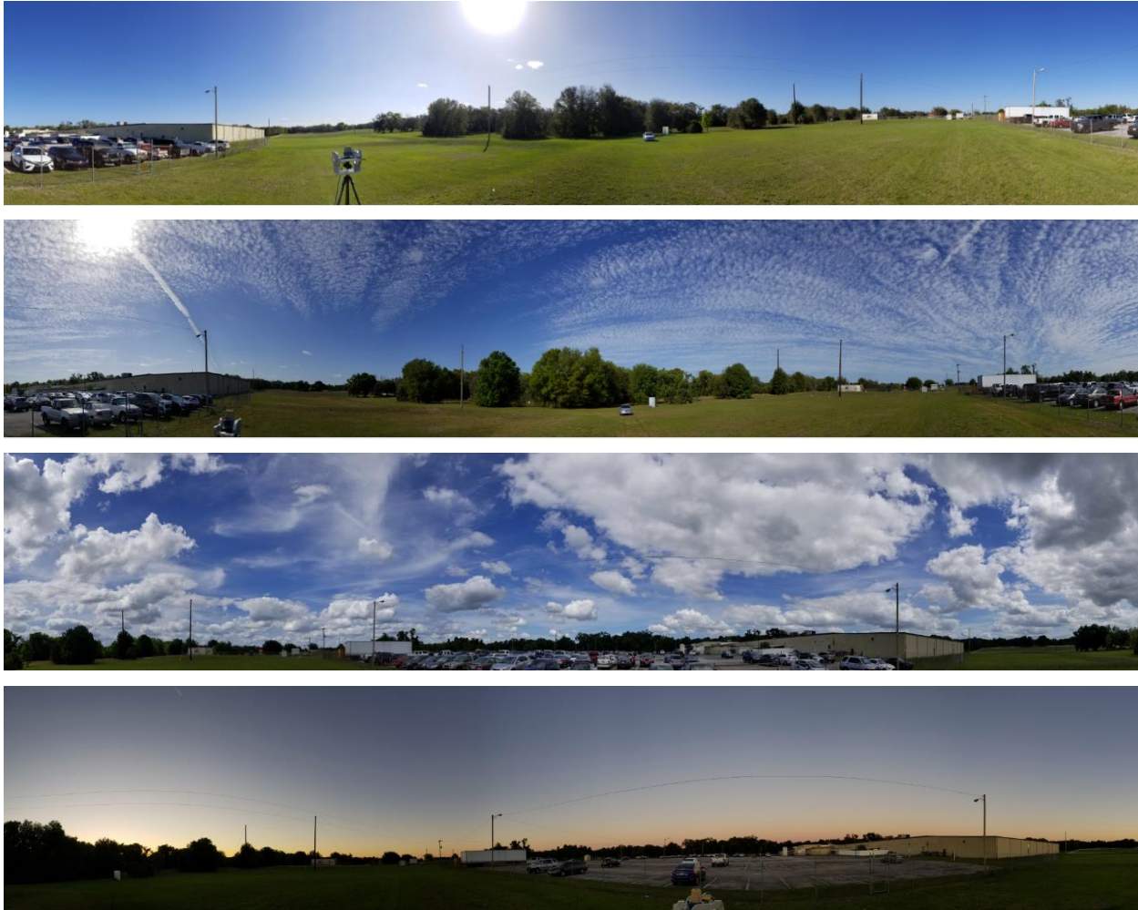
Figure 7. Example of clear skies (top), partial cloud cover (middle-top), heavy cloud cover (middle-bottom), and twilight (bottom) test conditions.
