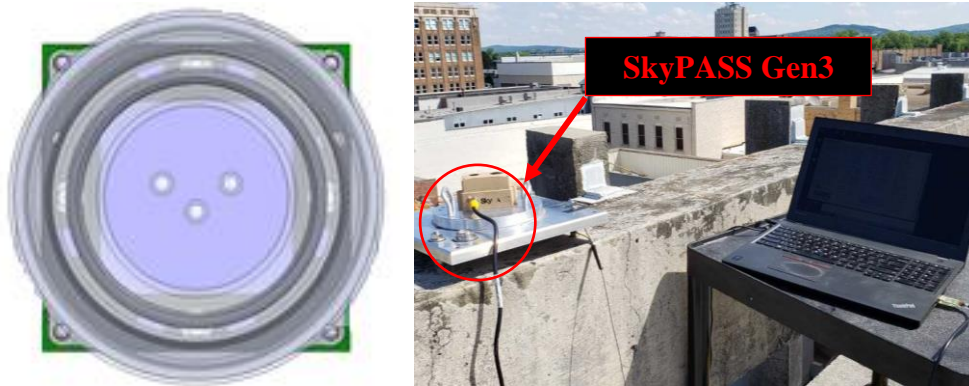
Figure 5. The SkyPASS polarimeter opto-mechanical design (left) has a size and weight of 1.5" x 1.5" x 1.2" and 1.76oz, respectively. When included with a sun tracker, embedded processing, and ruggedized housing (Gen3), the SWaP becomes 3.5" x 1.9" x 2.4", 8oz, and 4.1W, respectively. The performance of the SkyPASS polarimeter is characterized using a surveyed rotation plate.
